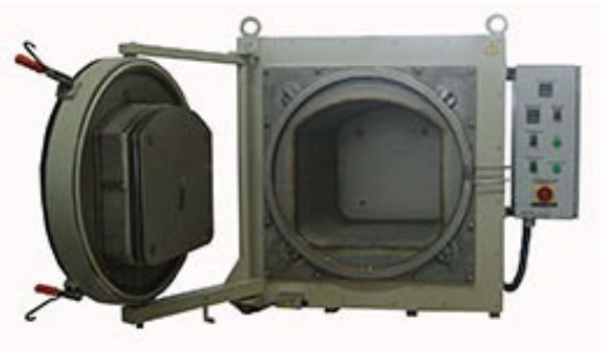
HCV CCH Controlled atmosphere From 3L to 1200 litres Temperature 1150°C
