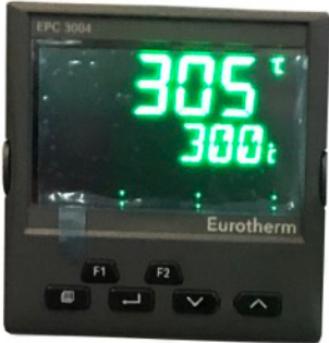
Eurotherm EPC3004 10 progs - 25 segments Suitable for Vacuum and controlled atmosphere furnaces Ethernet connection
