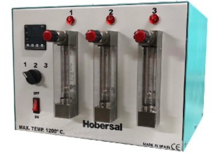
Gas supply system 1 Automatic flow meters
