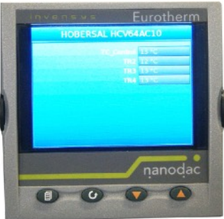
Eurotherm Nanodac Programmer/Recorder 100 progs - 25 segments According AMS2750 and 21CFR Ethernet connection USB
