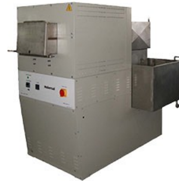
HB Series (static) Tempering and annealing Fast cooling 1150°C
