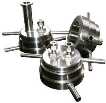
SS high vacuum end seals ( water refrigerated) high density, gas inlet and outlet, vacuum entry KF( x10-5) and thermocouple slot
