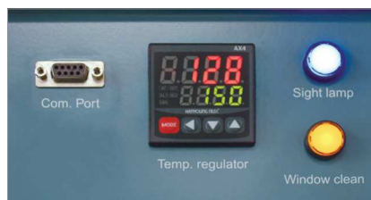
Electronic over temperature shutdown system.
