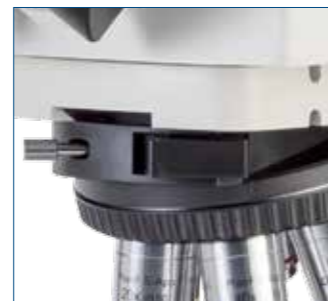
For slider with 1λ retardation plate for observation of monosodium crystal deposition (gout) and for DIC slot (DIC ready)
