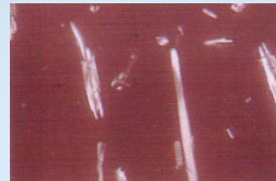
An unprocessed dispersion with a starting size range of 10-100microns (600X magnification).
